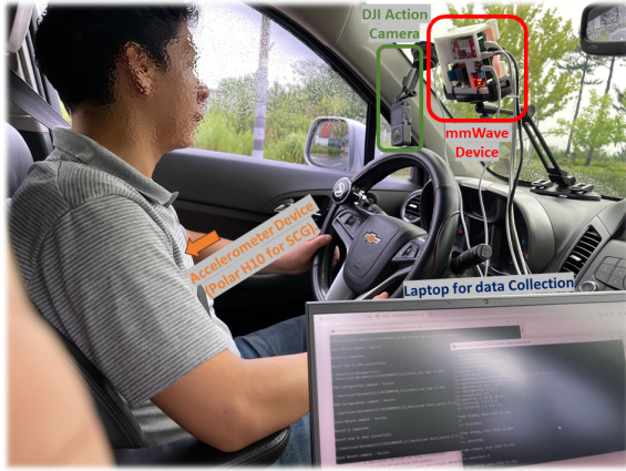
Figure 2: Car testbed setup: (a) mmWave device linked to laptop via Ethernet for vital sign capture; (b) Front glass-mounted video camera for facial expression capture; and (c) Polar-H10 device for acceleration-based heart rate and breathing capture.
