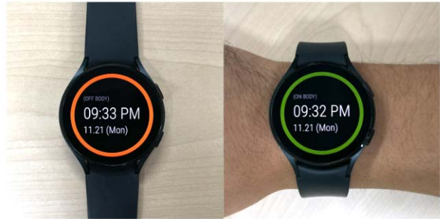
Fig. 1. Smartwatch data collection app while collecting sensing data. Application detects and marks data as off-body whenever wearable is not worn, and alerts user via color-coded UI.
