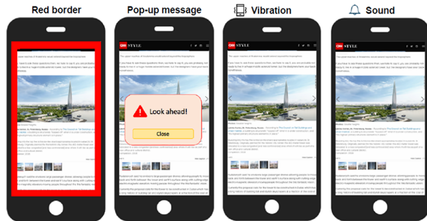
Fig 1. Four types of alert mechanism. Based on the results of our user study, we chose the two most preferred features (colored border and vibration) for the design of our app.
